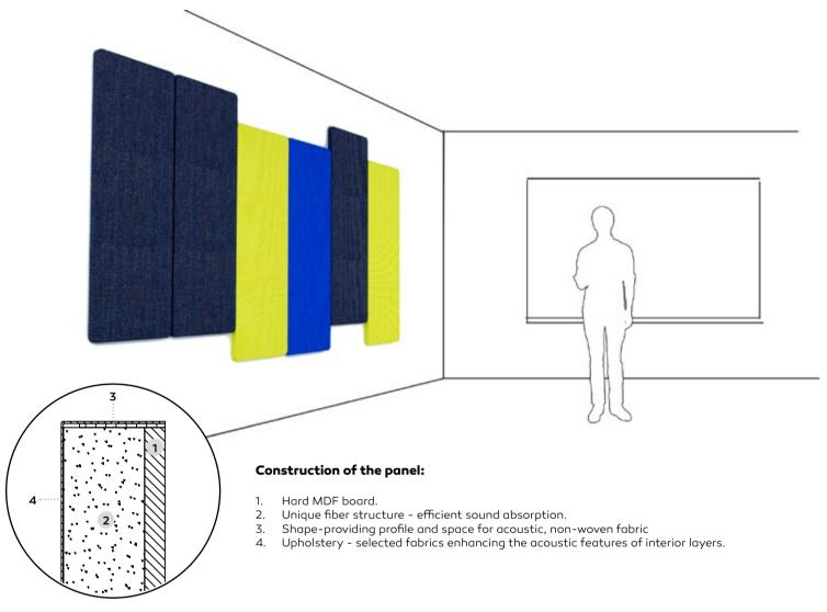
A cross-section of the Selva Wall acoustic panel
